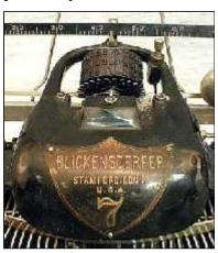
Instead of the common mechanism with letters on the end of individual bars connected to the keys, the Blickensderfer used a cylindrical wheel with letters embossed on it. Pressing a key caused the
