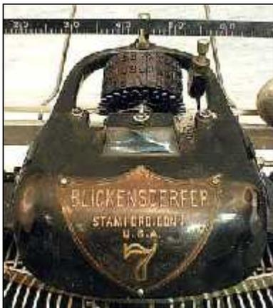
Instead of the common mechanism with letters on the end of individual bars connected to the keys, the Blickensderfer used a cylindrical wheel with letters embossed on it. Pressing a key caused the
